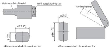
(Recommended dimensions for mounting the rotating shaft>
