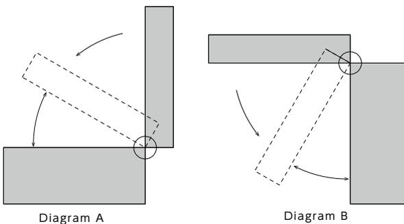
The damper torque becomes larger, preventing the lid from slowing down.
