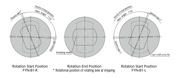
6. The direction in which torque is generated varies according to the model. Please select the appropriate model for your purpose.
