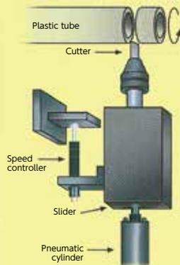
Precisely adjusting the cutting and feeding speeds in accordance with the materials and works is required. The speed controller can easily control the different feeding speed in accordance with the materials. Due to this, a standard pneumatic cylinder can be applied for structuring an inexpensive system in accordance with the materials.
