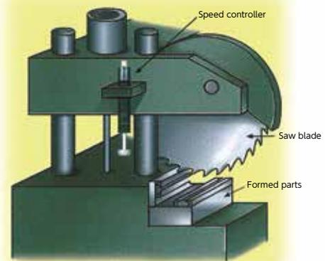
The saw blade will wear with the high cutting resistance of materials, such as aluminum and plastics. If the cutting is continued with this feeding speed, the saw blade or the material will be damaged. The attached speed controller on the tool head will provide the ease of feeding speed control to prevent the breakage, and the ease of mounting, which offers a low cost solution.
