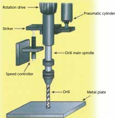
If the control of feeding speed is not possible at drilling, the excessive force will be applied to the drill, and the drill will bite into the work to generate a sharp projection and break the drill. By mounting a speed controller, the feeding speed of the drill can be precisely controlled to reduce burrs and remarkably reduce the breakage of drill.
