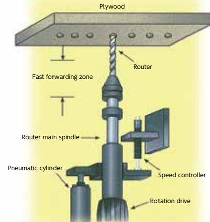
A custom-made tandem type pneumatic cylinder can provide the control of the fast forward and the low speed feeding at cutting. However, the mechanism becomes sophisticated, and the adjustment and the controllability do not perform optimally. By mounting a speed controller, the feeding speed can be precisely controlled; therefore, the equipment using a high cost custom-made tandem pneumatic cylinder can be replaced by a standard product.
